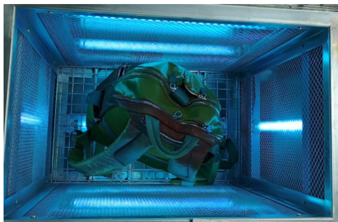
Powerful Ultra Violet UVC lamps kill viruses in seconds. This is a picture made on purpose, to show how it works. In real operation it is not possible to see the light if the cover is open.
