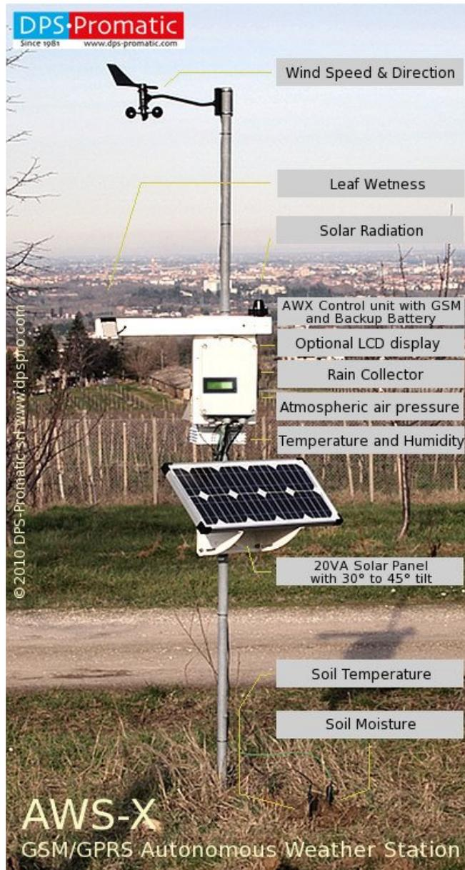
**AWS-X GSM/GPRS weather station**
